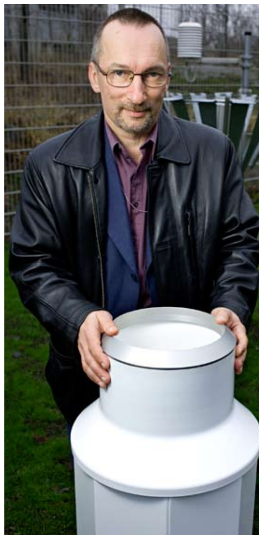
Keijo Leminen presenting an automatic precipitation sensor. Behind, a rain gauge of an old model.
